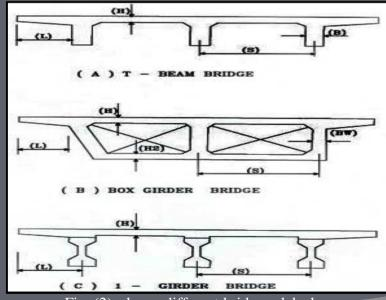
Fig. (2). shows different bridges slab shapes.
